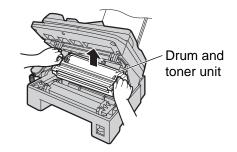
Turn the two levers on the used toner cartridge firmly.
